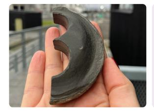
On top of the reservoir is a sealing layer of more than 100 meters of this caprock which ensures CO<sup>2</sup> containment.
